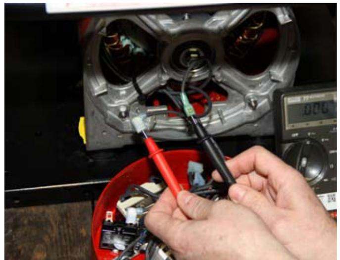
10. If you read the proper voltage output from the stator leads and you did not read the same voltage from the receptacles, then your losing voltage somewhere in the receptacle assembly. Check for loose wires, defective receptacles or defective circuit breakers. Replace defective parts as necessary and re-assemble. Test output after repairs are made.
