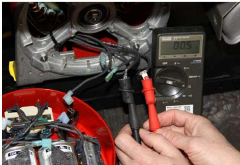
5. Check for continuity between the capacitor leads and the power output leads G-1 and G-3.
