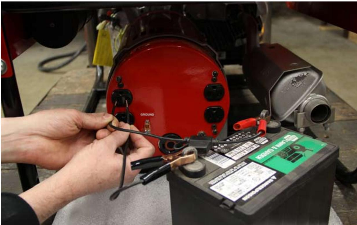
4. Re-check for output on all receptacles. If you read 120 VAC Line to Neutral on the 120 volt receptacles and 240 VAC Line to Line on a 240 volt receptacles you have successfully flashed the field.
