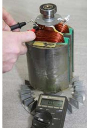
4. Check rotor leads for continuity and grounding. Place meter leads on solder end of diode(s). At least one of the diodes must be disconnected from the rotor to check continuity and resistance. There should be continuity between the leads and no reading to ground (metal shaft). The expected resistance values are listed in the table at the end of this guide. If rotor is out of specification or is grounded replace the rotor.
