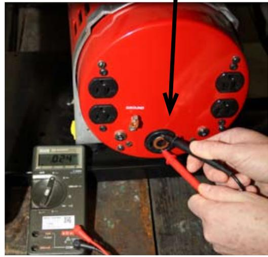
5. STOP the engine. You should be able to operate your generator normally at this time. If you do not read nominal voltage on the receptacles you will have to check for voltage at the stator leads of the generator.
