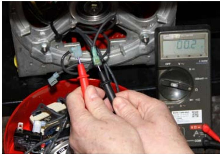
3. Check stator capacitor leads for continuity, resistance and grounding. Set your VOM to read Ohms resistance.
