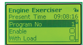
Fig. 13: Programmable Engine Exerciser
